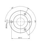
70 W continuous program power capacity 110 dB sensitivity 1200 - 20000 Hz response 1" horn throat diameter 38 mm (1.5 in) aluminum voice coil Annular HT polymer diaphragm
